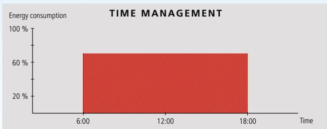
The light fittings are switched on continuously in the production hall during the entire operating time.
