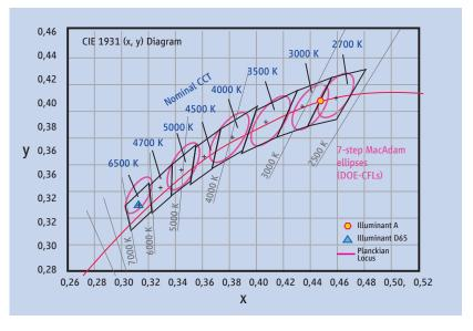
ellipse. Care should be taken to ensure small colour differences – especially for lighting applications where individual light sources are not far apart and can be seen simultaneously.
