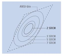
The colour coordinate tolerance of light sources is thus assessed using the steps of MacAdam ellipses (also referred to as SDCMs – Standard Deviations of Colour Matching). For compact fluorescent lamps, for example, international standards recommend a tolerance of at most a 7-step MacAdam ellipse (synonymous with 7 SDCM). From 3 SDCM upwards, differences are perceptible between colours at the edge of the ellipse and the colour at its centre.
